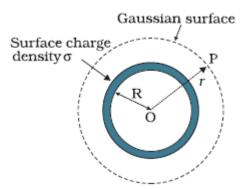
Electric flux through Gaussian surface
